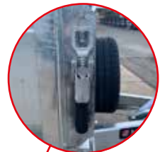
'Silent Sides': Spring loaded flip latches on all drop sides prevent undue movement and noise
