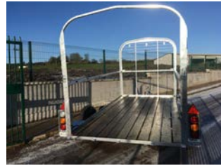
33mm preserved timber floor with aluminium treadplate for a fully sealed finish.
